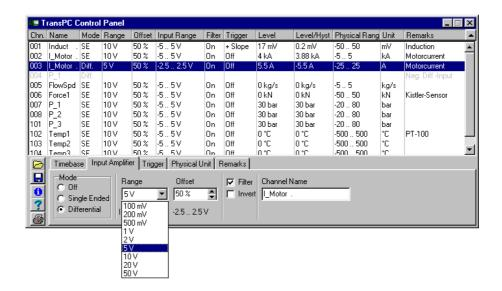
Clearly, a highly flexible measurement system with potentially high channel count requires an appropriate method of setting up the hardware.
