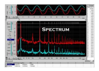
Sometimes it is necessary to convert time signals into the frequency domain. **TransCom-CompactX** performs this task using a fast Discrete Fourier Transformation.
