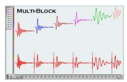
A series of bursts can be captured with minimum dead time between blocks.
