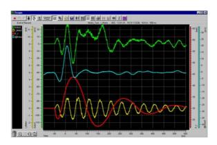
Single transients or repeated events are both displayed in scope mode. The captured signals are stored in the Transient modules independent of the PC memory, and can be displayed directly after capture.
