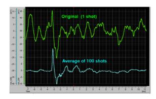
Averaging a signal over several triggered captures increases the signal to noise ratio making the desired signal more apparent.
