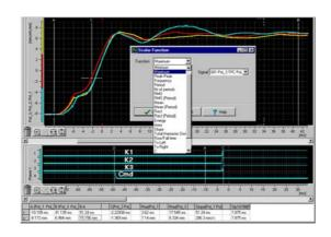
Signal scaling, labelling and grids are automatically optimised to match the selected portion of the signal trace.
