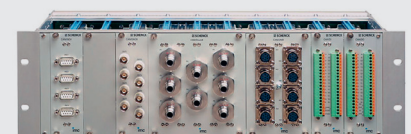
19" subrack for mounting of cassette type imc CANSAS modules: Backplane mainframe for user-configurable plug-in of modules with automatic slot recognition
